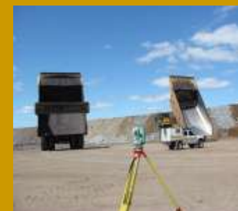
Measuring trucks to estimate the quantity of coal they can carry
