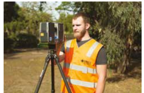
Student using a Trimble/Faro 3D laser scanner to measure the exterior of a building.
